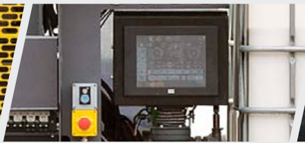
Redundant and single point control panel for all functions and operation overview.
