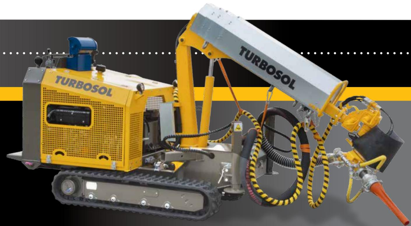
**TURBOSOL TSR 7. UNITÉ À CHENILLES POUR LES APPLICATIONS DU BÉTON PROJETÉ. AUTONOMIE TOTALE DU MOUVEMENT**
